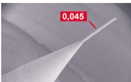
Micro pin structure in hard metal, length 1 mm
