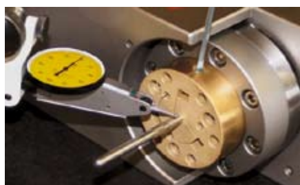
Adjustment of radial run-out with Adjustable Clamping Element H5.83.46R..
