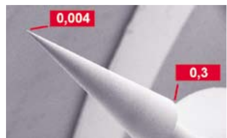
Stainless steel needle for medical technics, Ra 0.2 - 0.25 µm
