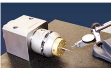
Presetting with Presetting Spindle and Adjustable Clamping Element
